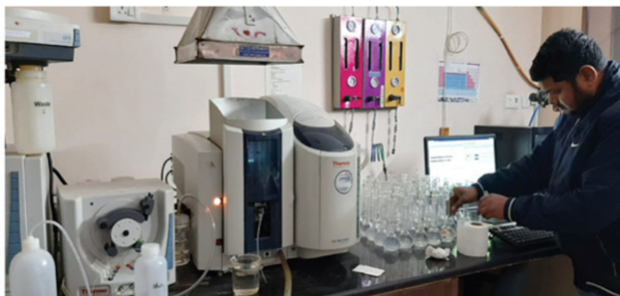
Analysis of Heavy metals using Atomic absorption spectrophotometer (AAS)
