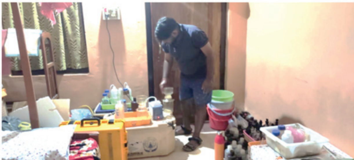
Filtration of water samples using vacuum pump in field
