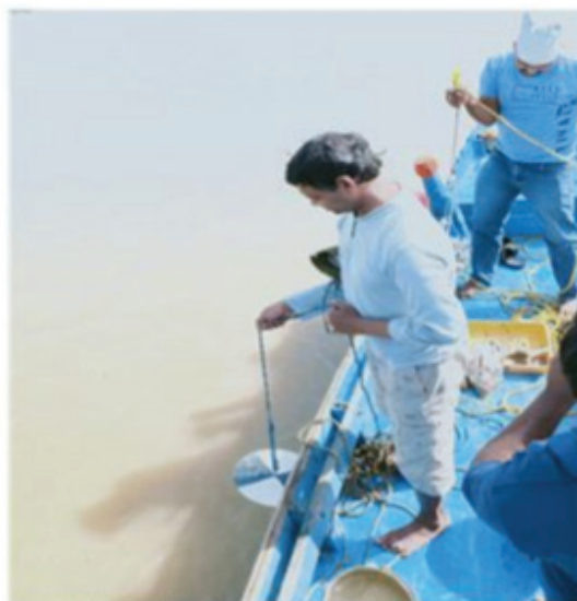
Measuring the depth and transparency by Secchi disc
