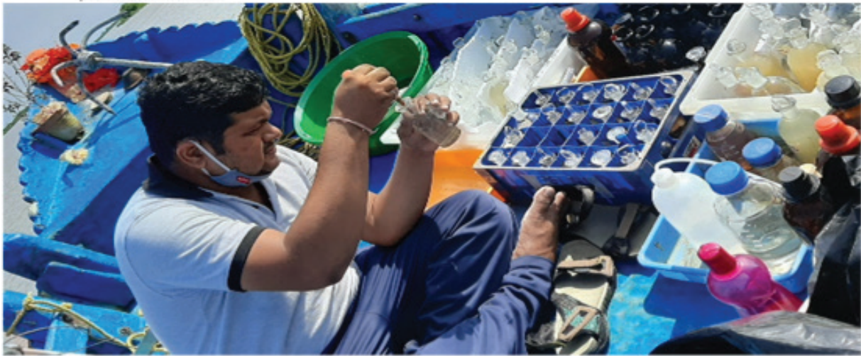
Fixing of DO samples immediately after collection
