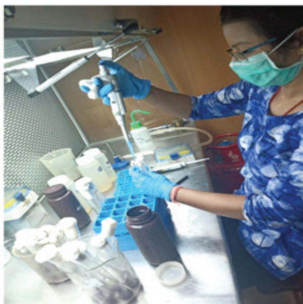
Performing the presumptive test for FC analysis
