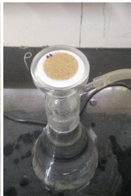
Figure 47 Sediment trapped on filter paper (45 microns) after filtering of a water sample
